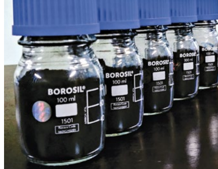
Graphite can be split into high-quality graphene (black powder in bottles) with a plasma spray technique.
