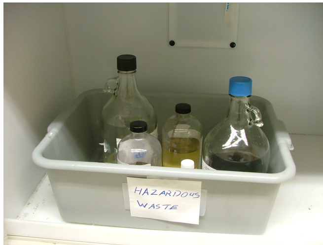
5. Example of a Satellite Accumulation Area. This one is located under the hood in S410 lab.
